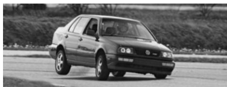
Shift of traction and vehicle balance from entering a turn too fast.
